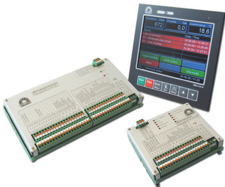
MEC24 monitoring and control panel, providing real-time alarm, safety and automated control functions with plain text alarm display on a 5.7" colour screen
