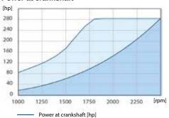
Power at calculated propeller load exp 3
