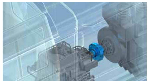
RENK diaphragm couplings are applied in locomotives and motor coaches
