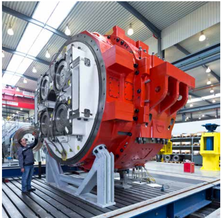
Assembling the world's biggest planetary gear system designed for the megasized wind energy nacelle testing unit at Clemson University, USA. The picture above shows the four planetary stages.
