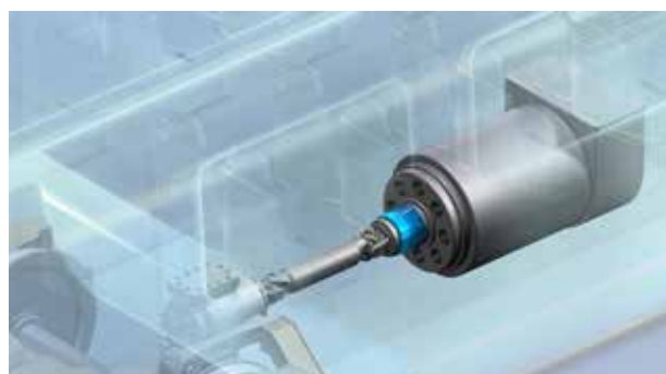
Drive unit of a high-speed train
