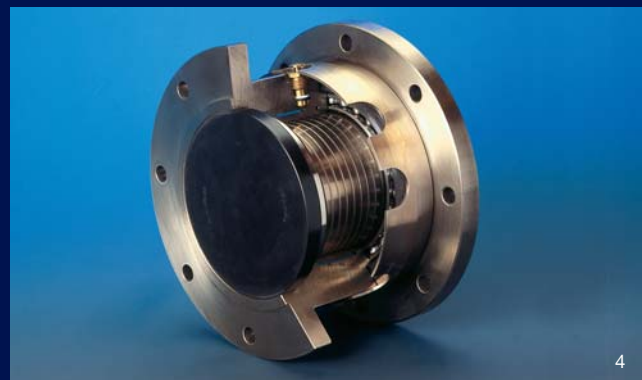
1 Curved Tooth Coupling with hardened and ground inner and outer teeth, tooth-by-tooth injection lubrication
