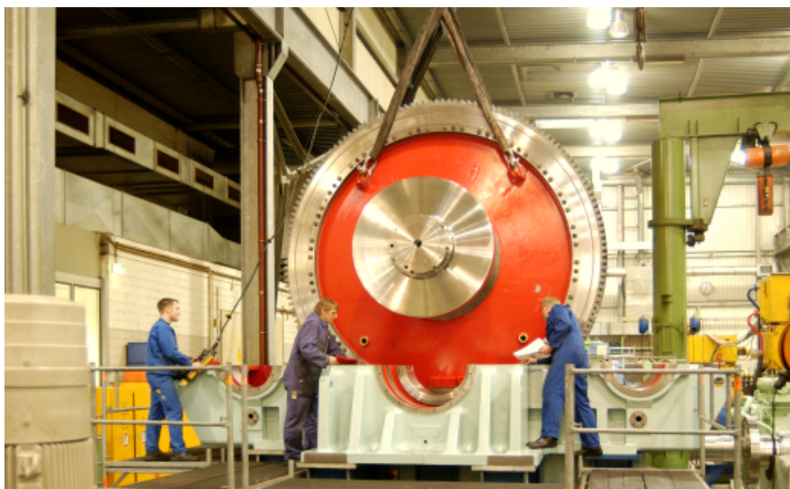
Installing the big wheel (diameter around 3,600 mm) of an NDSH-4000 double marine gear unit for a BP LNG tanker
