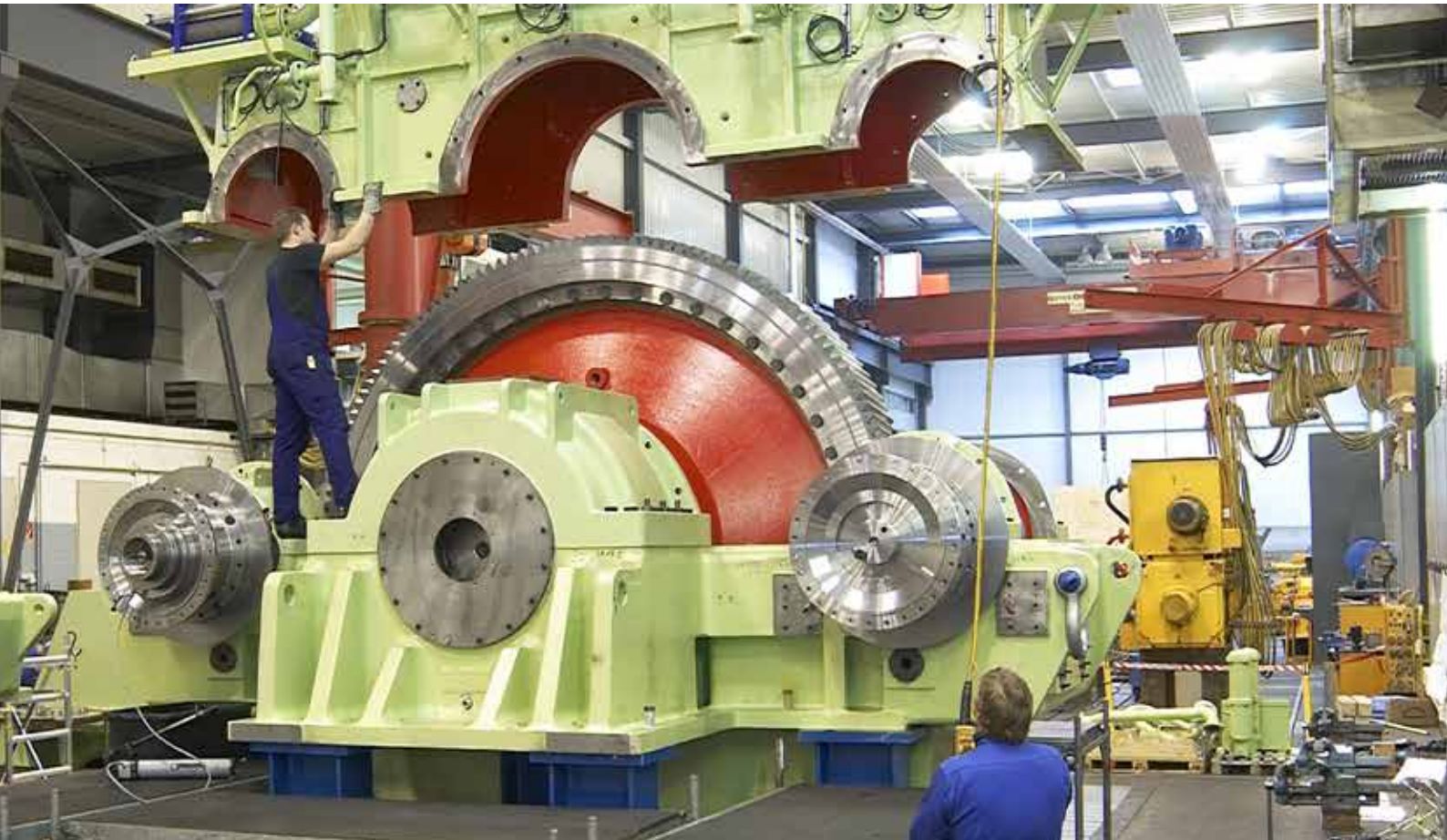
Assembly of an NDSH-3920 double marine gear unit
