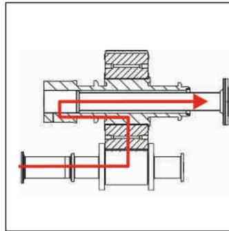
The quill shaft design takes advantage of the higher resilience of a long shaft, whereby the power flow is directed into the output shaft that is located opposite to the driven machine.
