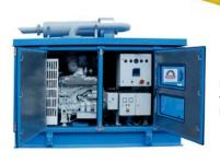
Marine Generating Set inside weather proofed canopy for installation on upper deck.
