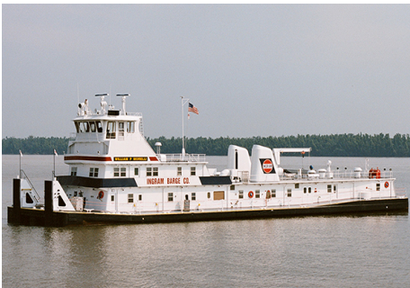
INGRAM BARGE COMPANY M.V. Mark Duley 2 x GE 8L250MDC (Mechanical Propulsion) Inland Marine Tow Boat
