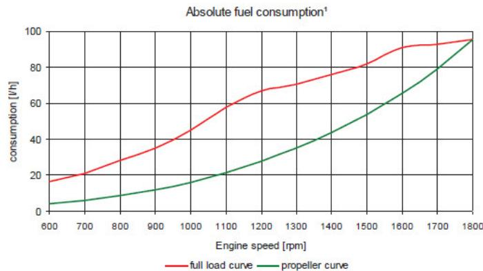
The rated power is based on reference conditions according to DIN ISO 3046 - 1 (2002) Exponent for propeller curve 2,7
