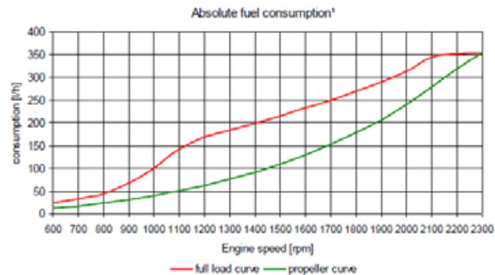
The rated power is based on reference conditions according to DIN ISO 3046 - 1 (2002) Exponent for propeller curve 2,5
