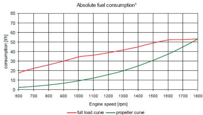
The rated power is based on reference conditions according to DIN ISO 3046 - 1 (2002)
