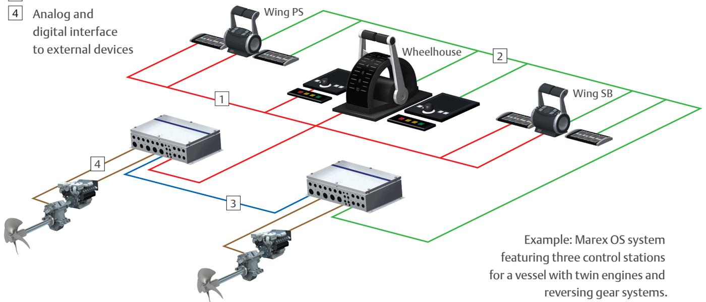
Example: Marex OS system featuring three control stations for a vessel with twin engines and reversing gear systems.
